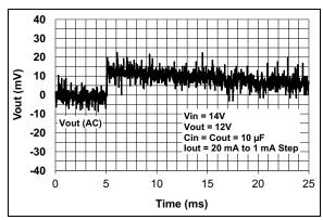
FIGURE 2-13: 12V LDO Dynamic Loadstep - Falling Current.
