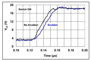
FIGURE 2-18: Buck Snubber Turn On.
