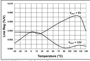
**FIGURE 2-1:** LDO Line Regulation vs Temperature.
