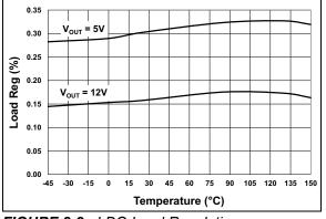
**FIGURE 2-2:** LDO Load Regulation vs Temperature.
