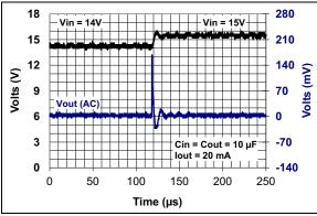
**FIGURE 2-8:** 12V LDO Dynamic Linestep - Rising  $V_{DD}$ .
