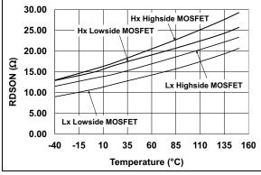
**FIGURE 2-20:** Gate Driver RDS<sub>ON</sub> vs Temperature.
