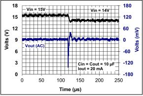
**FIGURE 2-9:** 12V LDO Dynamic Linestep - Falling V<sub>DD</sub>.
