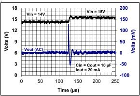
**FIGURE 2-6:** 5V LDO Dynamic Linestep -Rising V<sub>DD</sub>.
