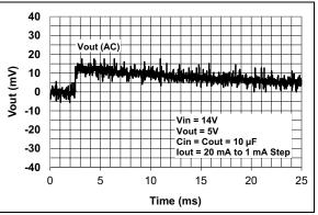
FIGURE 2-11: 5V LDO Dynamic Loadstep - Falling Current.
