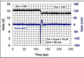
**FIGURE 2-7:** 5V LDO Dynamic Linestep - Falling V<sub>DD</sub>.
