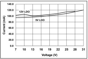
**FIGURE 2-5:** LDO Short Circuit Current vs Input Voltage.
