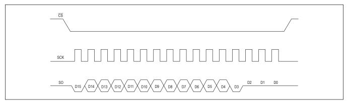
Figure 1a. Serial Interface Protocol
