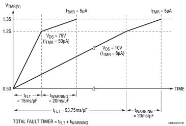
Figure 1. Overvoltage Fault Timer Current
