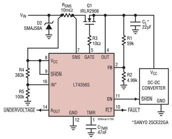
Figure 9. Overvoltage Regulator with Low-Battery Detection
