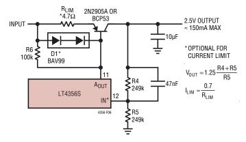
Figure 6. Auxiliary LDO Output with Optional Current Limit
