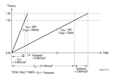
Figure 2. Overcurrent Fault Timer Current
