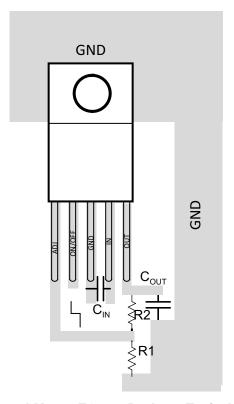
Figure 22. LM2941 TO-220 Package Typical Layout
