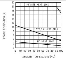
Figure 17. Maximum Power Dissipation (TO-220)
