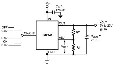
$V_{OUT} = Reference \ voltage \times \frac{R1 + R2}{R1} \ where \ V_{REF} = 1.275 \ typical Solving for R2: R2 = R1 \left( \frac{V_O}{V_{RFF}} - 1 \right)$
