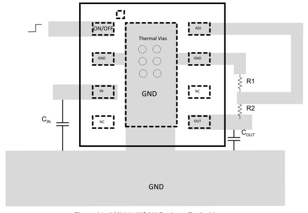
Figure 21. LM2941 WSON Package Typical Layout
