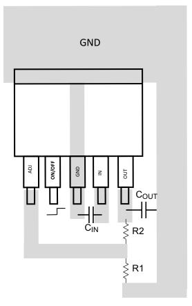
Figure 23. LM2941 TO-263 Package Typical Layout
