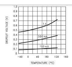
Figure 1. Dropout Voltage
