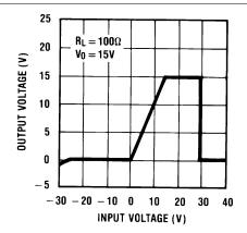
Figure 14. Output at Voltage Extremes
