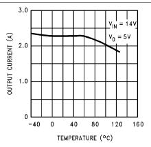
Figure 15. Output at Voltage Extremes
