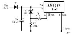
Figure 27. Undervoltage Lockout Without Hysteresis for an Inverting Regulator
