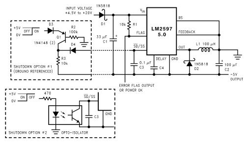
Figure 24. Inverting –5-V Regulator With Shutdown and Soft-Start
