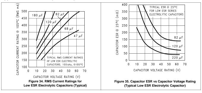
The consequences of operating an electrolytic capacitor above the RMS current rating is a shortened operating life. The higher temperature speeds up the evaporation of the electrolyte of the capacitor, resulting in eventual failure.
