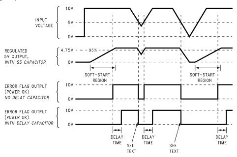
Figure 33. Timing Diagram for 5-V Output
