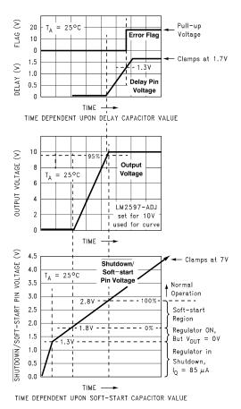
Figure 31. Soft-Start, Delay, Error, and Output
