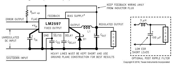
Component values shown are for  $V_{IN}$  = 15 V,  $V_{OUT}$  = 5 V,  $I_{LOAD}$  = 500 mA
