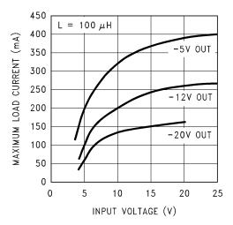
Figure 25. Maximum Load Current for Inverting Regulator Circuit
