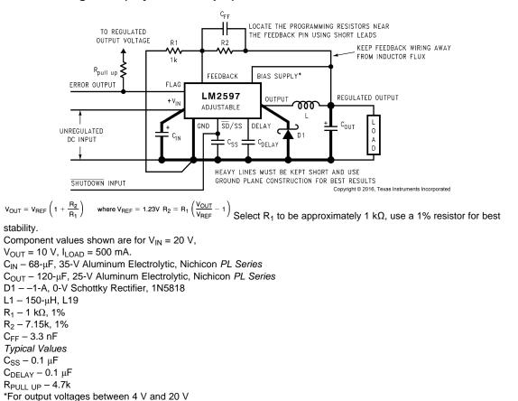
Figure 46. Adjustable Output Voltage Versions
