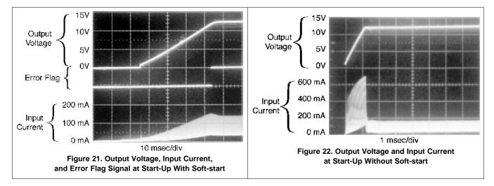
This reduction in start-up current is useful in situations where the input power source is limited in the amount of current it can deliver. In some applications, soft start can be used to replace undervoltage lockout or delayed start-up functions.
