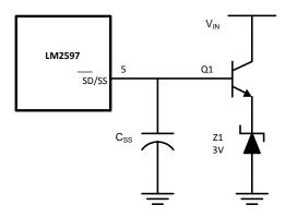
Figure 32. External 3.7-V Soft-Start Clamp
