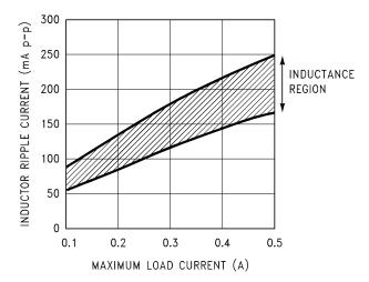
Figure 42. Peak-to-Peak Inductor Ripple Current vs Load Current
