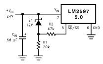
Figure 26. Undervoltage Lockout for a Buck Regulator
