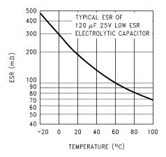
Figure 36. Capacitor ESR Change vs Temperature
