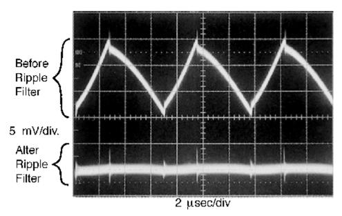
Figure 30. Post Ripple Filter Waveform
