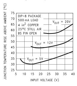
Circuit Data for Temperature Rise Curve
