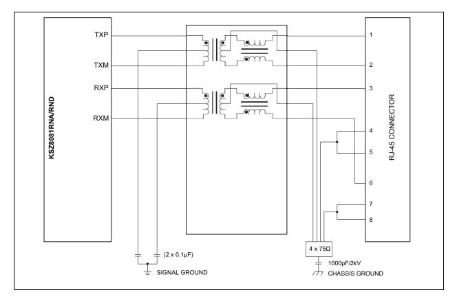
FIGURE 11-1: TYPICAL MAGNETIC INTERFACE CIRCUIT
