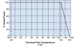
For resistors operated at a terminal part temperature of described for each size or above, a power rating shall be derated in accordance with the above derating curve. Please refer to "Introduction of the derating curve based on the terminal part temperature" in the beginning of our catalog before use.
