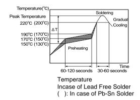
[Allowable Reflow Soldering Temperature and Time]
