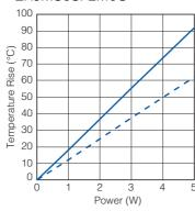
Base material : FR-4 (t1.6mm) Copper Thickness : 70 µm, Two layer
