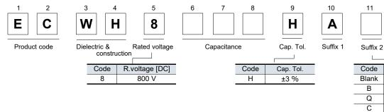
Rated voltage 800 V (Odd size taping)
