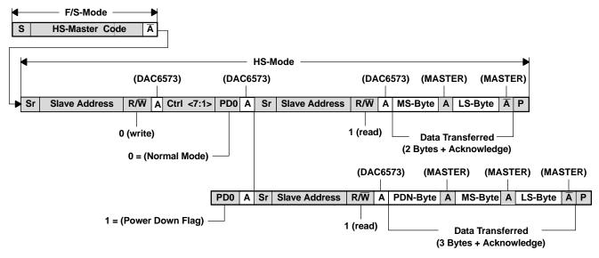
Figure 36. High-Speed Mode: Slave Transmitter
