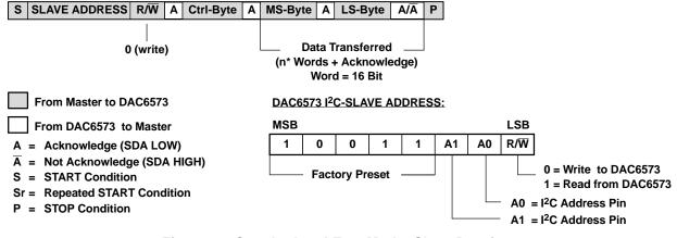
Figure 33. Standard and Fast Mode: Slave Receiver
