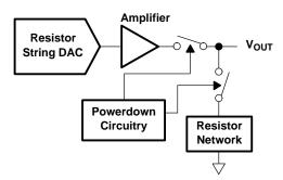
Figure 37. Output Stage During Power Down
