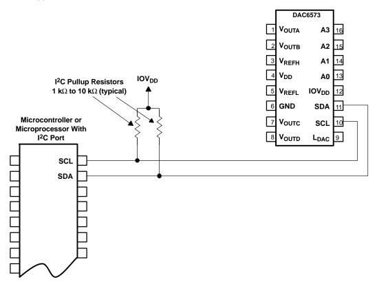
NOTE: DAC6573 power and input/output connections are omitted for clarity, except I<sup>2</sup>C Inputs.
