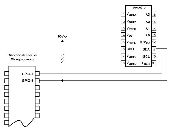
NOTE: DAC6573 power and input/output connections are omitted for clarity, except I<sup>2</sup>C Inputs.
