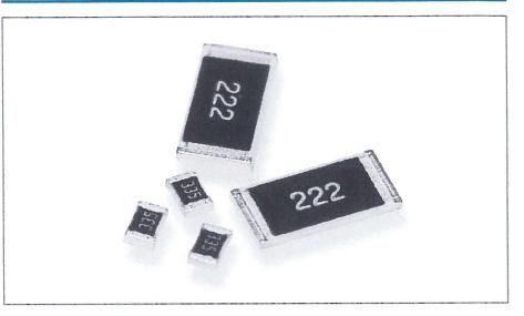
Precious metal terminations are screen printed onto a ceramic base and fired. The resistive element is screen printed and fired and the passivation layer added. Each resistor is trimmed to tolerance by laser. The pre-scribed tile is broken into strips, the end plating is fired on and the strips broken into individual components. Final termination is made by electroplating.
