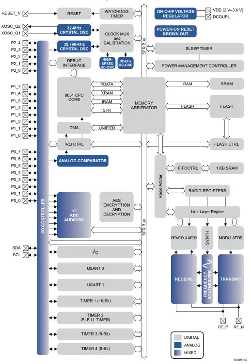
Figure 1-1. Block Diagram
