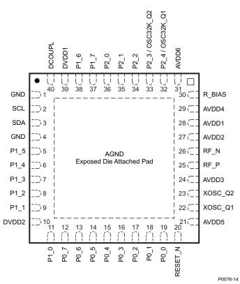
NOTE: The exposed ground pad must be connected to a solid ground plane, as this is the ground connection for the chip.
