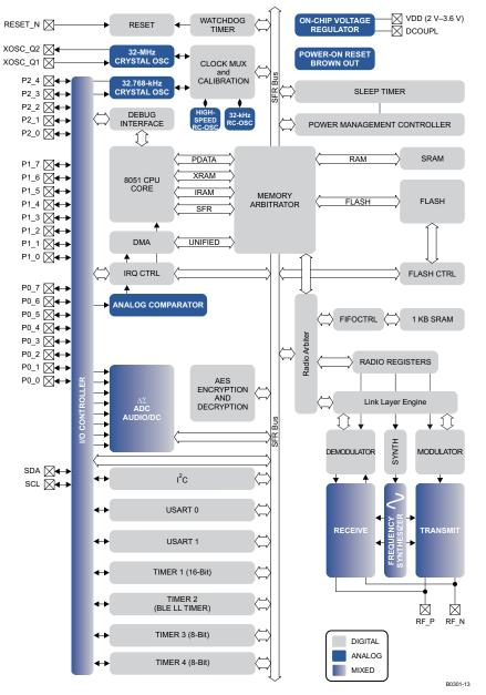
Figure 5-1. CC2541-Q1 Block Diagram
