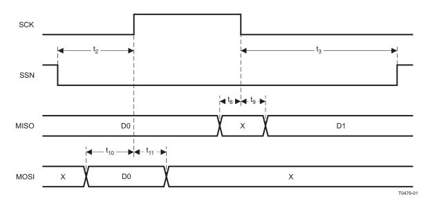
Figure 4-3. SPI Slave AC Characteristics
