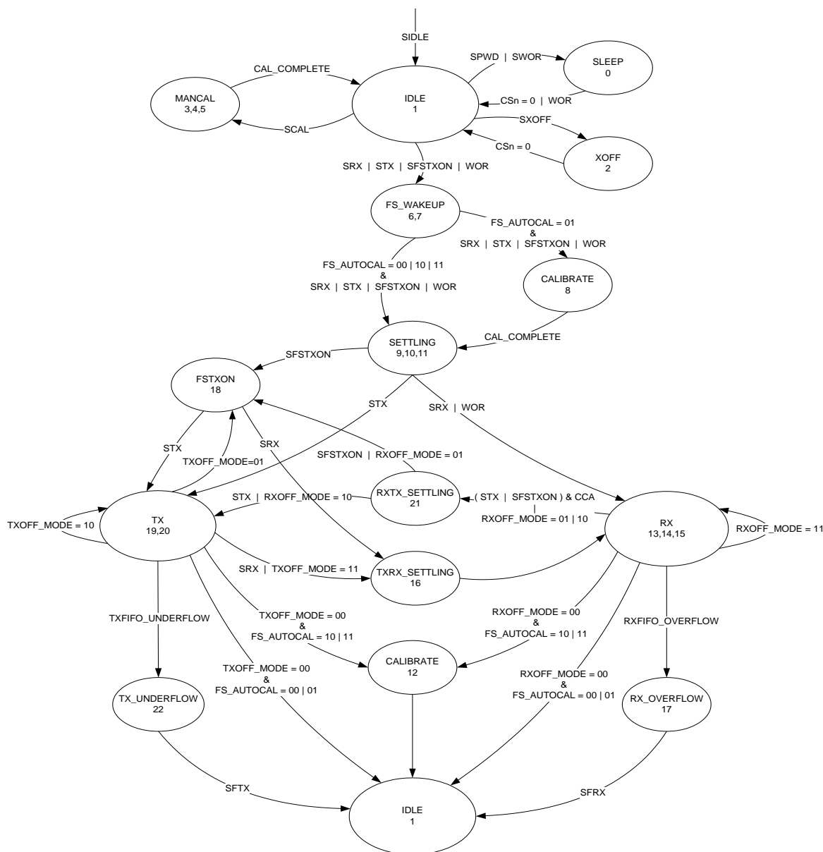
Figure 25: Complete Radio Control State Diagram
