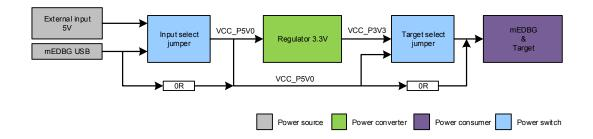
The input voltage select jumper (J300, 3-pin header footprint) can be soldered in to select between power from the USB port or from the VIN pin on the Arduino power header footprint. By default, the selector is bypassed with a  $0\Omega$  resistor (R300) to connect the USB voltage to the on-board 3.3V/150mA regulator and target voltage select header.
