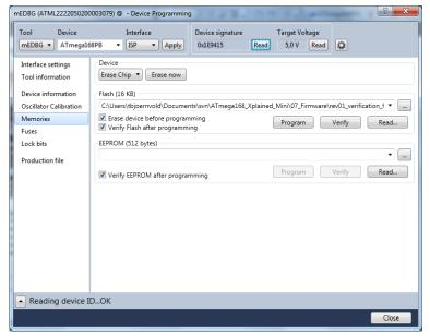
4. **NOTE:** If a previous debug session was not closed by selecting "Disable debugWIRE and Close" in the Debug menu, the DWEN fuse will be enabled and the target will still be in debug mode, i.e. it will not be possible to program the target using the ISP interface.
