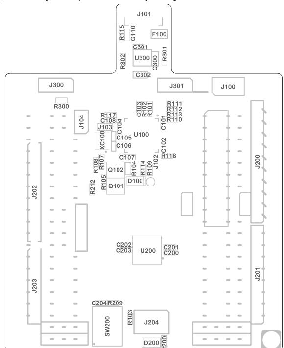
Figure 4-1. ATmega168PB Xplained Mini Assembly Drawing
