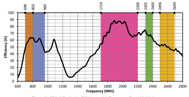
Figure 5. SP610 Radiation Efficiency with Frequency Band Highlights
