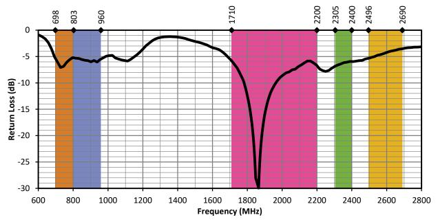
Figure 2. SP610 Return Loss with Frequency Band Highlights
