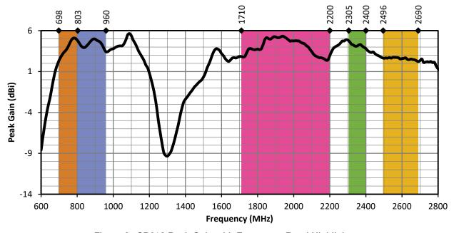
Figure 3. SP610 Peak Gain with Frequency Band Highlights
