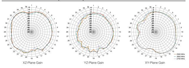
Figure 8. Radiation Patterns for the SP610 Antenna
