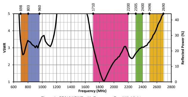
Figure 1. SP610 VSWR with Frequency Band Highlights
