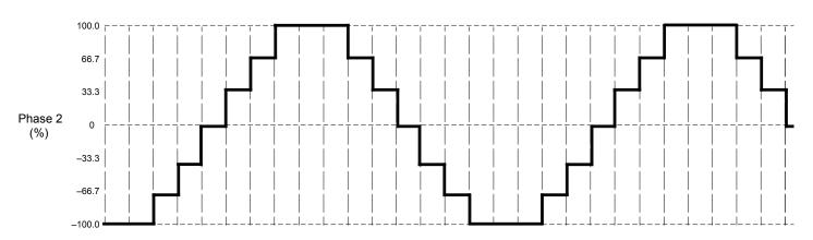
Figure 7. Step Sequence for Quarter-Step Increments
