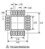
For Reference Only; not for tooling use (reference JEDEC MO-220WGGD)
