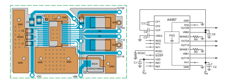
LP package typical application and circuit layout
