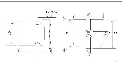
Unit: mm L +0.1 -0.4 Size W±0.2 H±0.2 C±0.2 øD±0.5 R P±0.2 code E7 8.0 8.3 9.0 6.9 8.3 0.6 to 0.8 3.2 F8 10.0 7.9 10.3 10.3 11.0 0.6 to 0.8 4.6 E12 8.0 11.9 8.3 8.3 9.0 0.8 to 1.1 3.2 F12 10.0 12.6 10.3 10.3 11.0 0.8 to 1.1 4.6
