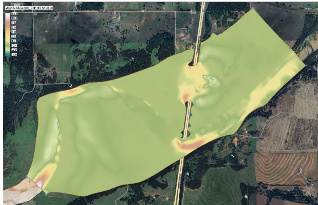
Figure 4 Erosion at the end of the unsteady flow sediment transport simulation
