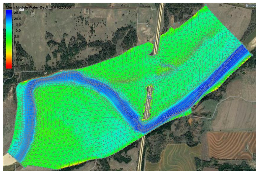
Figure 1 Flow depth on a dry mesh
