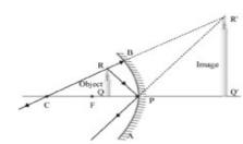
When the object is located between the focus (F) and the pole (P) of the mirror, the image is formed behind the mirror; this image is virtual, erect and large.
