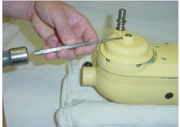
Fig. 67) Carefully drive the groove pin into the shaft of the planetary.
