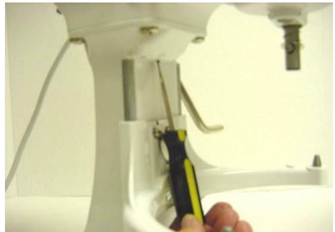
Fig. 96) Adjusting the beater to bowl clearance using the bowl height adjusting screw
