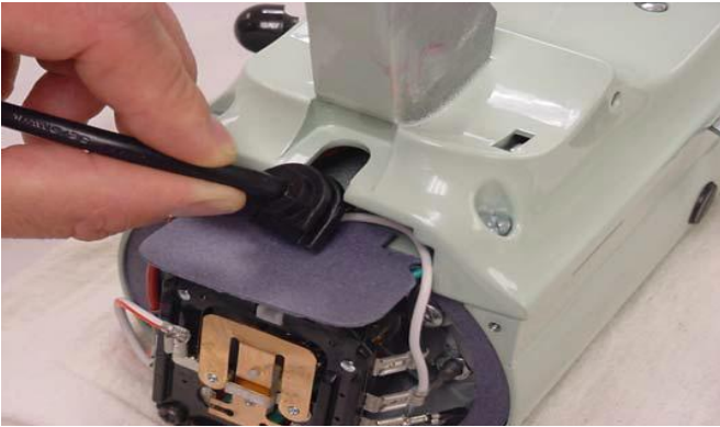
Fig. 11 Pull back on the molded strain relief to remove the power cord from the slot in the bottom cover
