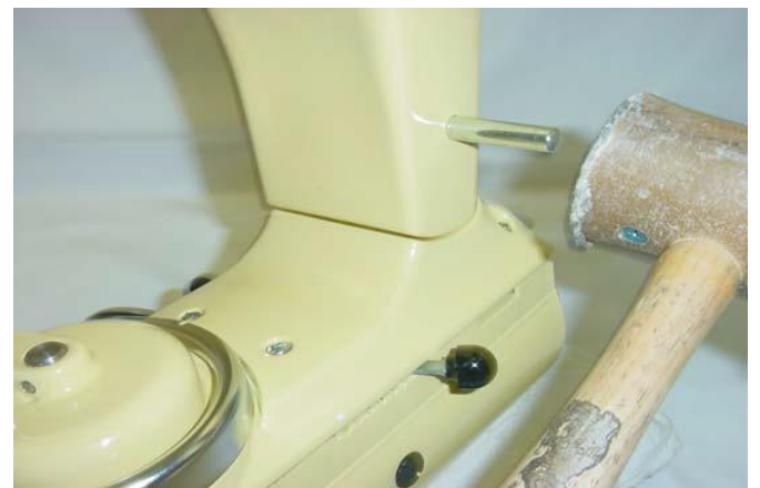
Fig. 72) Use a rubber or rawhide mallet to tap the hinge pin into the pedestal.
