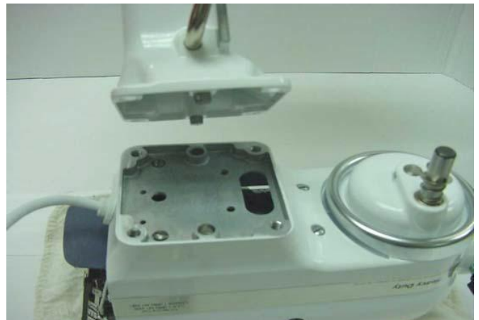
Fig. 84) Lift the column and bowl support assembly off of the bottom cover.
