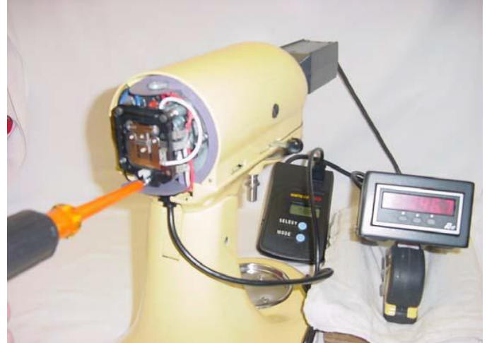
Fig. 79) Adjust the bottom speed setting screw for speed #2.
