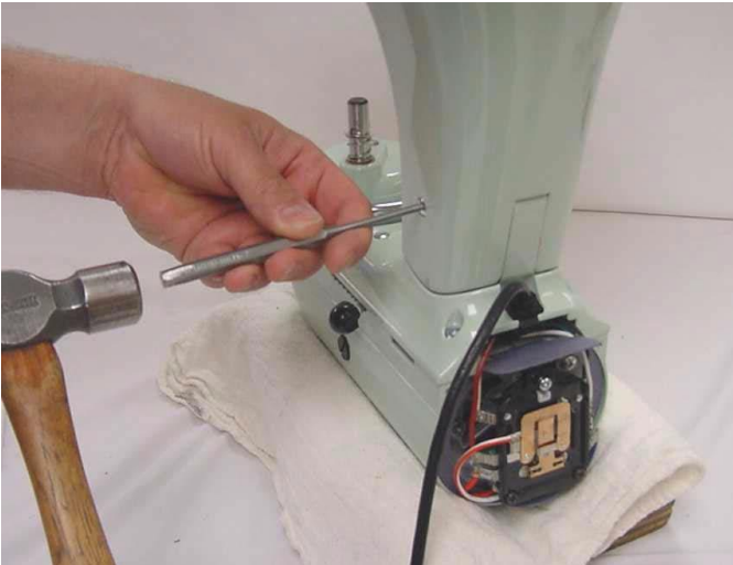
Fig. 7) Use a drift punch and hammer to drive out the hinge pin.
