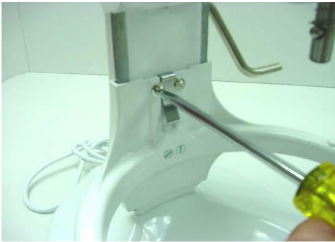
Fig. 94) Two #10-24 x 1/4" screws hold the bowl latch spring in place.
