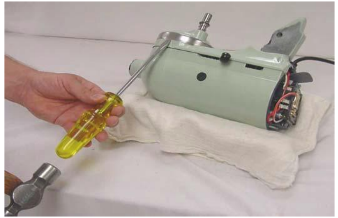
Fig. 8) The Drip Ring fits tightly and must be started off by tapping it.
