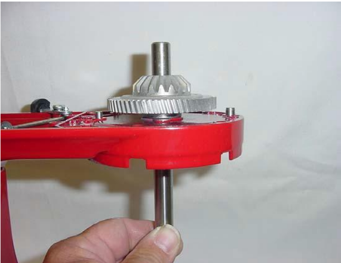
Fig. 54) Remove the (vertical) center shaft from the lower gear housing.
