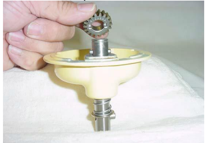
Fig. 64) Lift the pinion gear from the agitator shaft.
