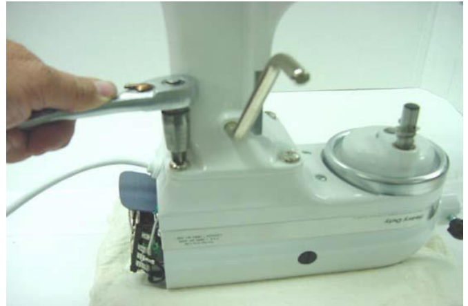
Fig. 83) Four round Phillips head screws must be removed to replace the bowl support assembly.
