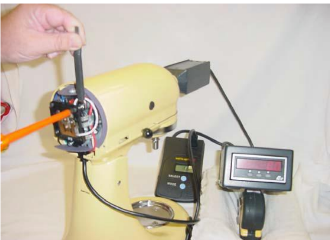
Fig. 78) Setting speeds using the digital tachometer.
