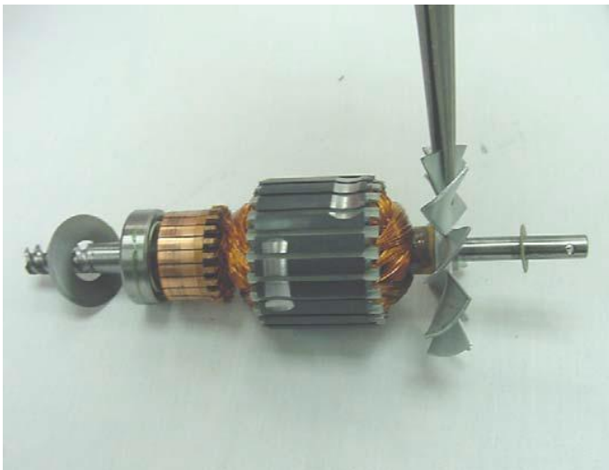
Fig. 40) Check the blades of the armature ventilating fan and straighten if bent.
