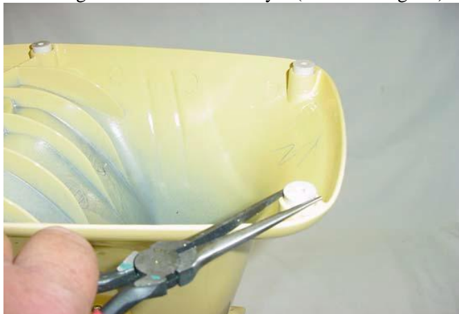
Fig. 70) The pedestal feet should be replaced on older mixers.
