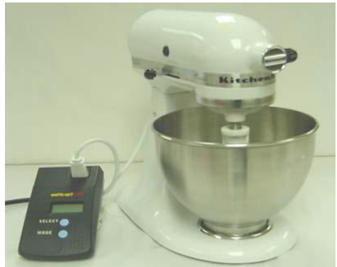
Fig. 3) KitchenAid stand mixer shown plugged into a digital wattmeter.
