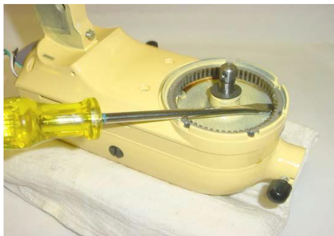
Fig. 60) Remove the internal gear by prying around and under its edge with a large flat blade screwdriver.
