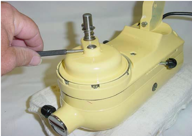
Fig. 66) A pointed punch can be used to align the holes of the shaft with the planetary.
