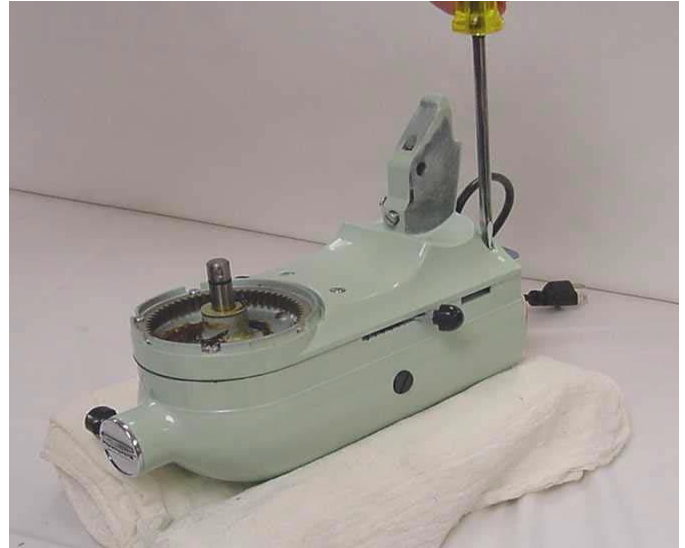
Fig. 14 Removal of the four #10-24 fillister head screws on an older unit with the slotted head screws.
