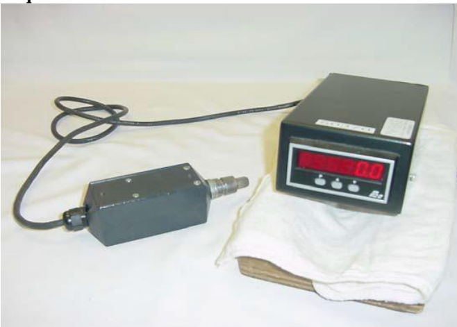
Fig. 77) Digital tachometer for setting speeds on KitchenAid mixers .
