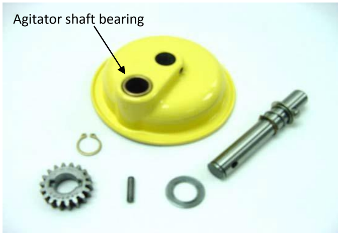
Fig. 65) disassembled planetary components.
