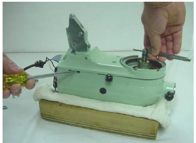
Fig. 15 While lifting up on the center shaft, use a screw driver to gently pry the bottom cover from the housing. Remove the attachment hub bevel gear from the gear case/motor housing.
