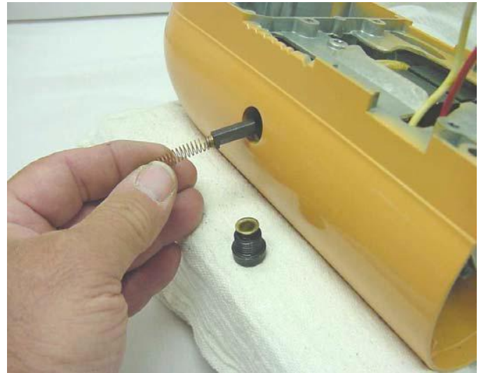
Fig. 31) The brush holder caps are loosened to access brushes for removal. Make sure to note brush orientation. The armature can now be removed.
