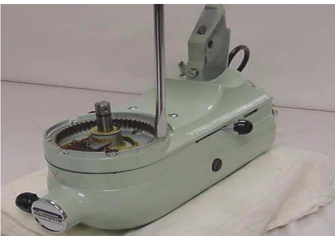
Fig. 13 Removal of the five #10-24 slotted flat head screws holding the internal gear in the bottom cover on an older model.
