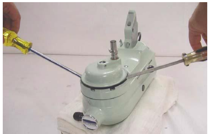
Fig. 10) Use two screwdrivers to pry the planetary off from the center shaft
