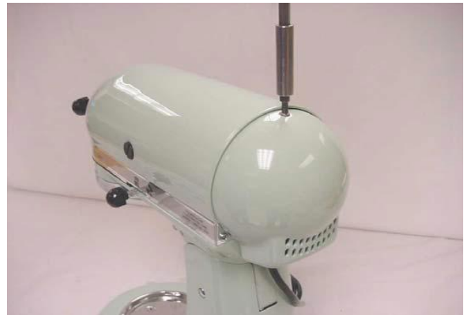
Fig. 4) Removing the tapered head end cover screw.
