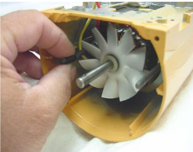
Fig. 30) The motor stud sleeve is shown being removed after bearing bracket removal.
