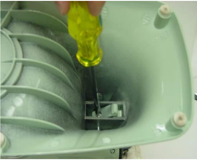
Fig. 6) Loosen the hinge pin setscrew to remove the pedestal from the bottom cover.
