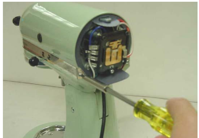
Fig. 5) Removing the trimband screws.
