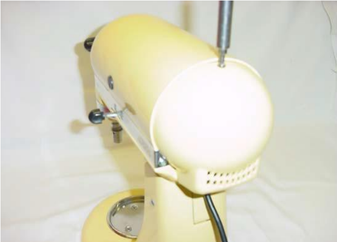
Fig. 81) Secure the end cover with a tapered head screw.
