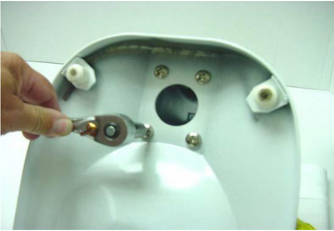
Fig. 85) Remove the four round head screws from the base to separate it from the bowl lift assembly.
