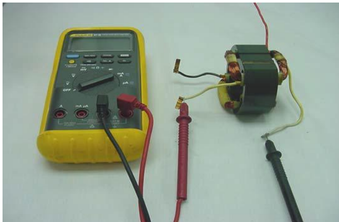
Fig. 37 Test the two stator coils for continuity with an ohmmeter set on the low ohms scale.
