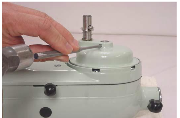
Fig. 9) Remove the groove pin that holds the planetary to the vertical center shaft.
