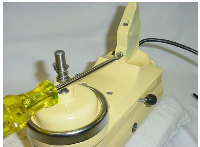
Fig. 68) The beater height adjusting screw has a nylon insert and should not be loose in the threads.
