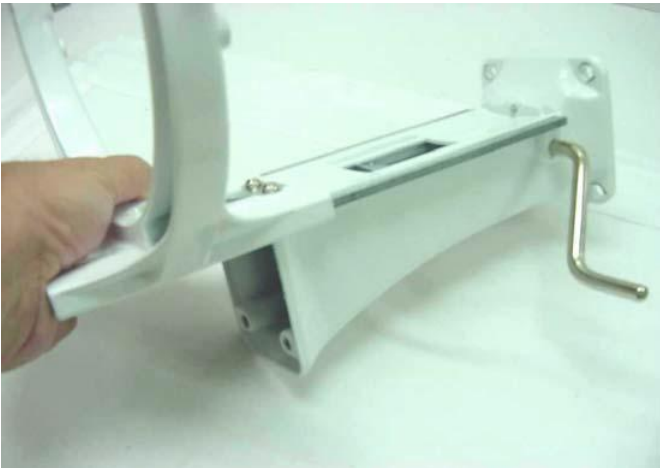
Fig. 87) Slide the bowl support down and off the column to access the bowl lift assembly.
