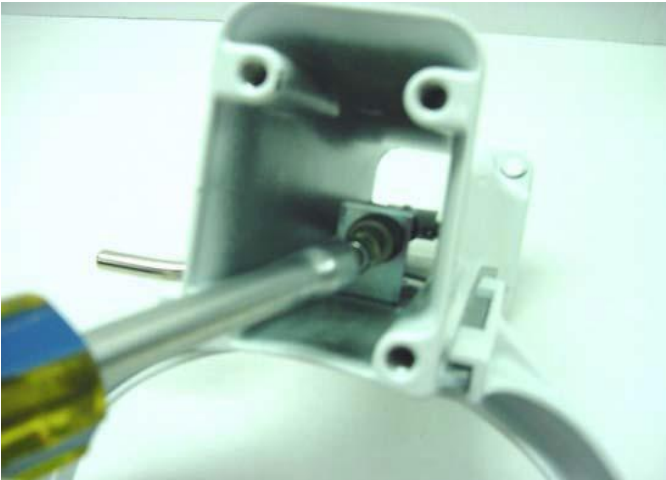
Fig. 91) Check the nut for proper tension on the bowl lift bracket.
