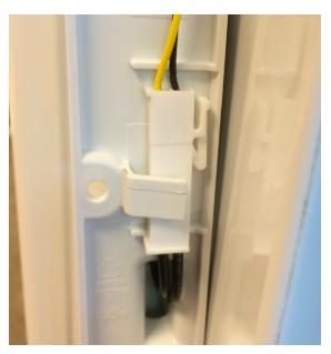
FIGURE 11: Mullion Heater Wiring Connector Routed Behind Clip
