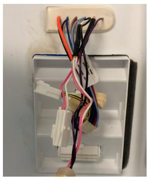
FIGURE 19: Smoke Staining Caused by Laser Cutting
