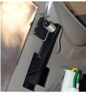
FIGURE 10: Ice Paddle Torsion Spring
