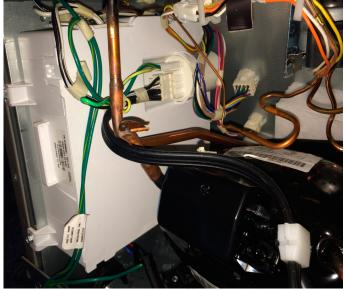
FIGURE 1: Orion Assembly with EMI Filter
