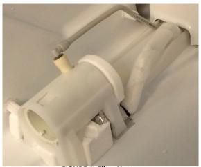
FIGURE 1: Filter Heater
