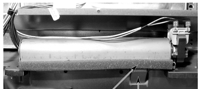
Foam Tape Over Air Duct Screw
