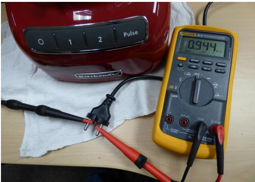
Safety Switch test measurement.
