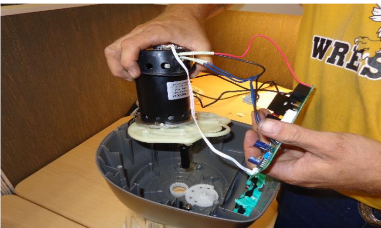
Fig. 12) Remove motor and control board together
