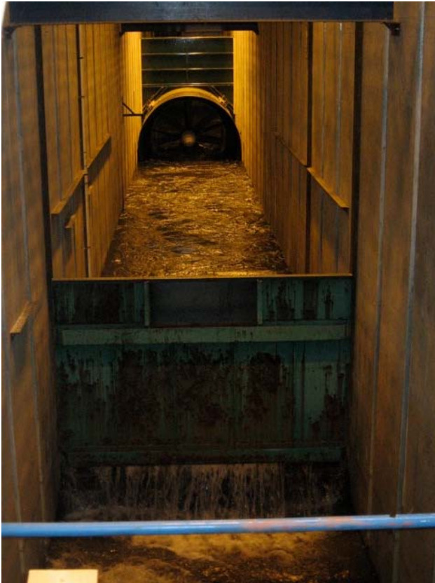
Turbine installed in 10 ft wide flume
