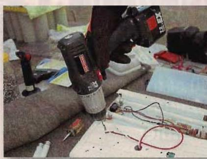
1) The ballasts covers on our Optronics were attached with small pop-rivets that needed to be drilled out.
