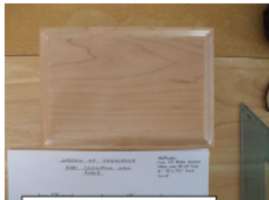
Cap with Miter Corners
