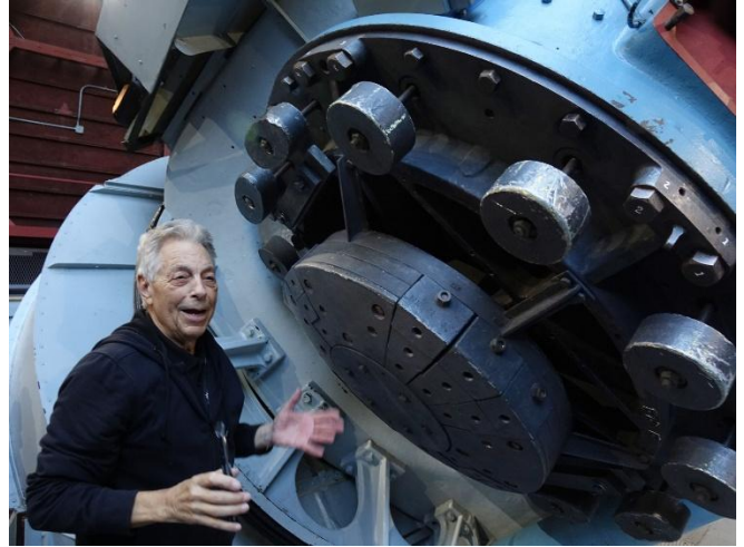
The big cylinder behind our guide, Tom, contains the mercury pool for the 60-inch telescope. The 100-inch telescope needs two such pools!
