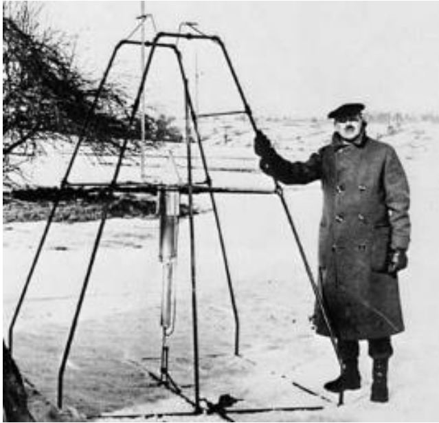
Dr. Robert H. Goddard and his liquid oxygen-gasoline rocket circa 1926, at Auburn, Mass. It flew for only 2.5 seconds, climbed 41 feet, and landed 184 feet away in a cabbage patch. Photo credit: NASA
