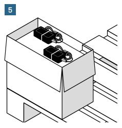
■ Place AC adaptors on top of cardboard sheet. Secure AC adaptors with tie wraps or bands.
