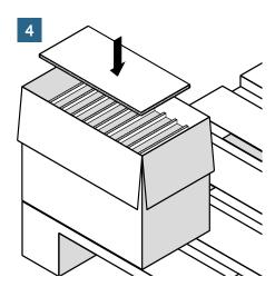
■ Leave spaces at the sides of the box for extra protection. Place cardboard sheet over the top.
