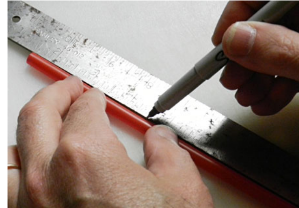
Figure 5. Marking a straight line down the length of the straw helps keep the joints lined up so the finger bends more naturally.
