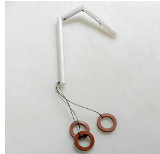
Figure 8. A finger with three joints and one tendon for each joint. Pulling a ring makes the joint it is attached to bend.
