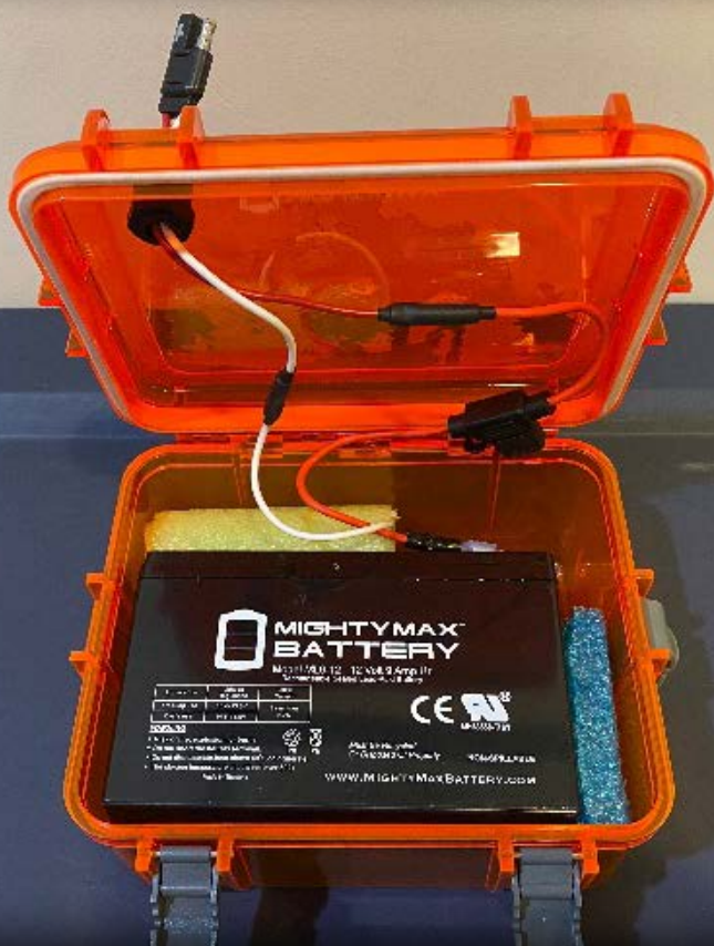
The author's watertight enclosure for his kayak's battery. The box size is larger than the battery itself, so pieces of pool noodle the battery from shifting inside the box.
