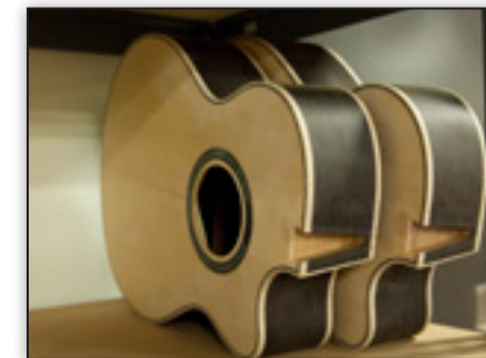
Collection Series II Acoustic bodies staged for neck and body assembly
