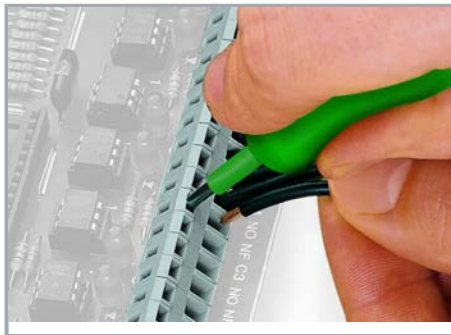
Inserting a conductor via 3.5 mm screwdriver.
