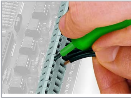
Inserting a conductor via 3.5 mm screwdriver.
