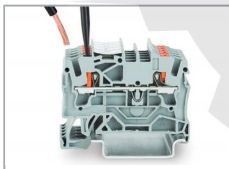
Insert fine-stranded conductors via operating tool.
