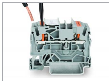
Insert fine-stranded conductors via operating tool.
