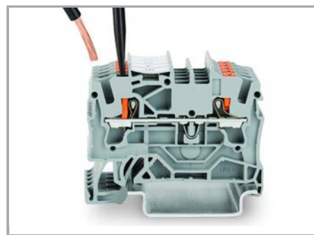
Insert fine-stranded conductors via operating tool.
