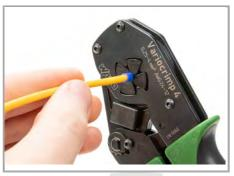
Squeeze handles until ratchet mechanism is released.
