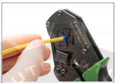
Squeeze handles until ratchet mechanism is released.
