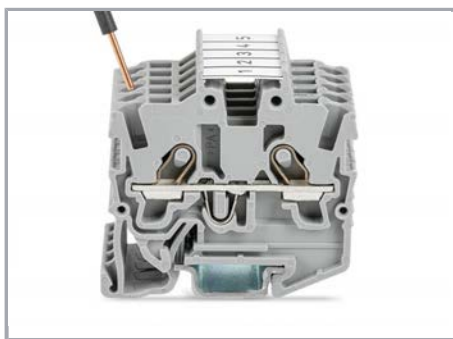
Insert solid conductors via push-in termination.
