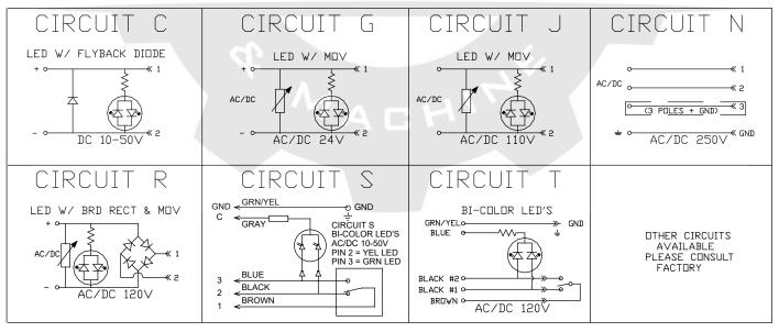
Valve Connectors with LEDs and surge suppression aides in diagnostics and protection of equipment.
