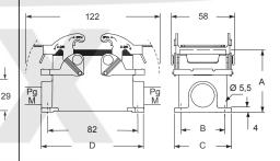
The lever, due to the vertical closing movement, offers an IP66/IP67/IP69 degree of protection (according to EN 60529) when fitted with a complete and coupled connector and used with ILME standard hoods in die cast aluminum with pegs (without adapter).
