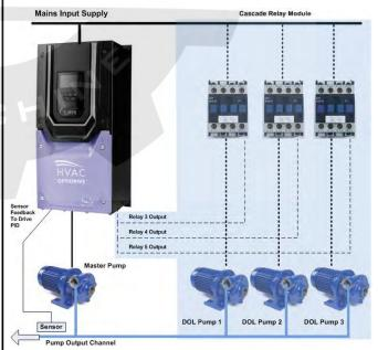
For this configuration only parameters P8-14 and P8-15 need be set and the relays in the cascade module are assigned automatically starting with the lowest numbered relay.
