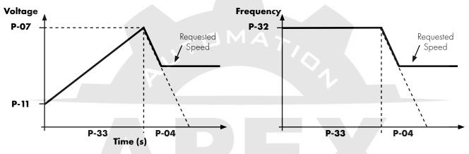
In order to achieve reliable starting and optimise the starting method, the following procedure can be used.
