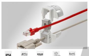
QVT-CLICK is a circular split frame for quick and easy installation of pre-terminated cables or complete cable harnesses. But also electric, pneumatic or hydraulic lines without terminals or connectors as well as corrugated conduits can be easily routed and sealed with IP54. Because of its extremely compact design, the QVT-CLICK range is especially suitable for small machines, devices and instruments.
