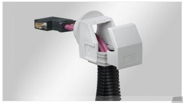
The split KVT-W90 cable glands are used to insert and seal pre-terminated cables at a 90° angle. But also electric, pneumatic or hydraulic lines without terminals or connectors as well as corrugated conduits can be easily routed (e.g. into control panels, enclosures or machinery) and sealed with IP54.
