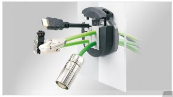
KVT-ER are split cable glands for routing and sealing cables with connectors, with diameters from 1 to 16 mm (KT 1 - 15) and 16 to 35 mm (KT 16 - 34). But also electric, pneumatic or hydraulic lines without terminals or connectors as well as corrugated conduits can be easily routed (e.g. into control panels, enclosures or machinery), sealed and strain relieved acc. to EN 62444.
