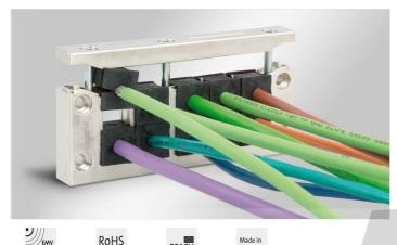
The EMC cable entry frames EMC-KEL-U are based on the KEL-U and KEL-E. Due to a conductive surface, disturbances in the cable shields on the control cabinet can be easily dissipated. Field bound disturbances are derived by the metallisation.
